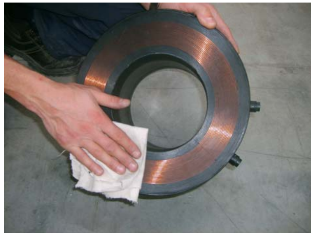
If it is necessary, EF Saddle must be cleaned with an appropriate chemical before welding.
